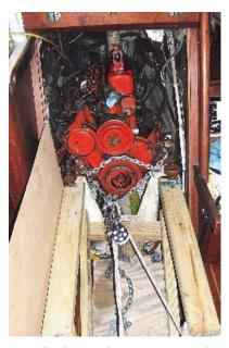
5. The engine will go though the companionway (just) without the transmission, alternator, and manifold. The new engine will just fit with removing nothing (it is a bit shorter, but really no different in the other dimensions). (See picture: Westerbeke out)
