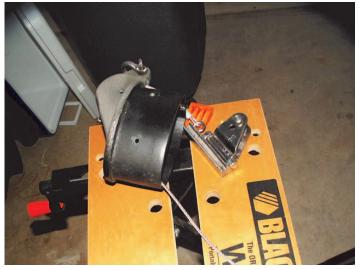
The outhaul consists of the outhaul car connected to a wire rope that connects to a block and tackle arrangement within the boom (two, two-sheave fiddle blocks) and then the line goes out through the forward end of the boom.
