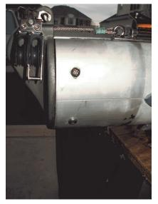
I used two techniques to loosen and remove the screws. I started with a large square-shafted screwdriver. I used an adjustable wrench on the square shaft to give me more torque. This technique only worked for some of the fasteners and a small vice grip was used to remove the
