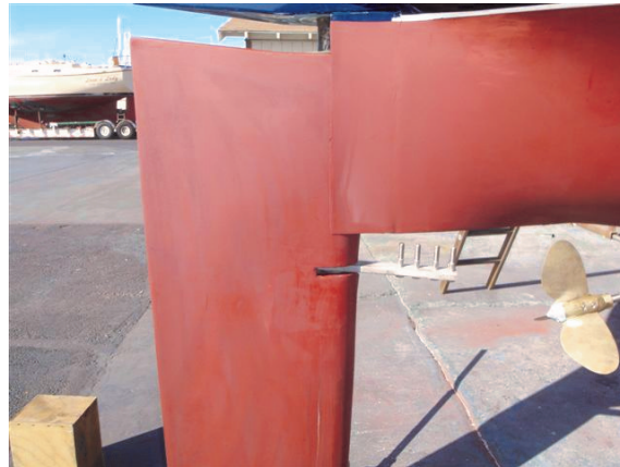
New pintle in place and plug epoxied back in rudder
