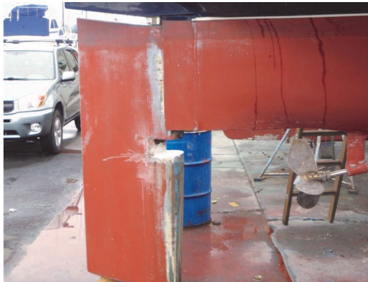
After cutting out the “plug” that holds the pintle in
